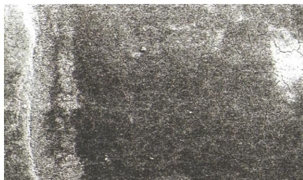
Fig. 9: SEM view of test side instrumented for 100 strokes with curette. 50x
