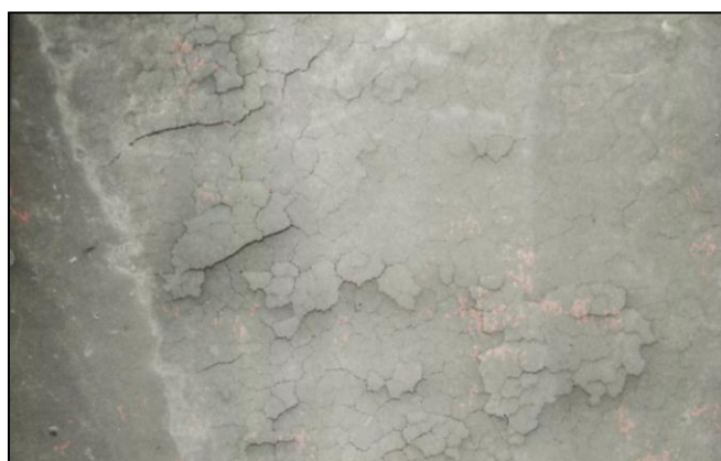
Fig. 15: SEM view of test side instrumented for 30 seconds with ultrasonic perio mini-tip. 50x magnification.
