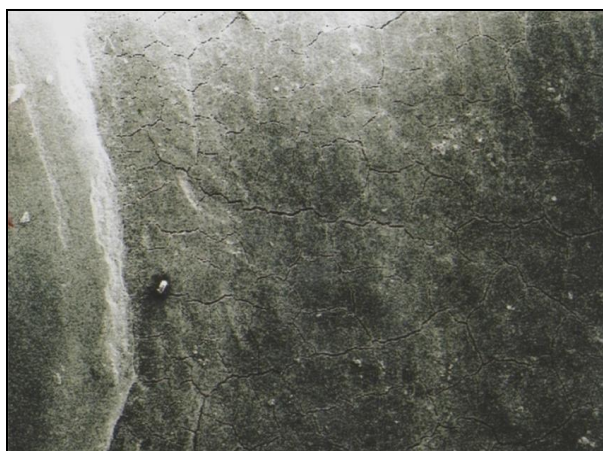
Fig. 16: SEM view of test side instrumented for 45 seconds with ultrasonic perio mini-tip. 50x magnification.
