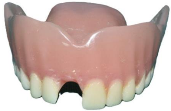
Figure 2: Debonding of denture tooth.
