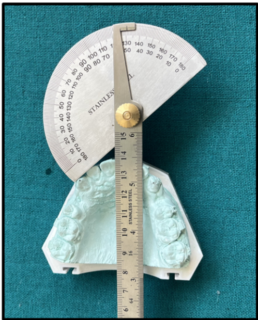
Figure 5: Measurement of rotation with protractor angle finder
