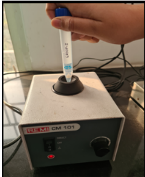
Fig. 2: Sample suspended in 5ml of physiologic saline and vortexed
